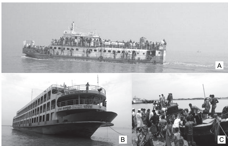
Figure 5: Different types of transport: A. Sea-truck, B. Launch, C. Engine propelled boat Source: Tasfin Aziz 2014
